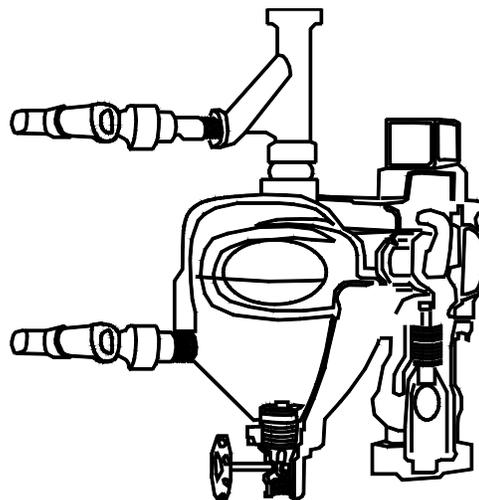
Figure 3. Combination LWFCO And Boiler Water Feeder.
