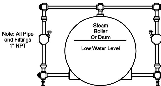
Figure 1. Typical Piping For Two LWFCO Units.
