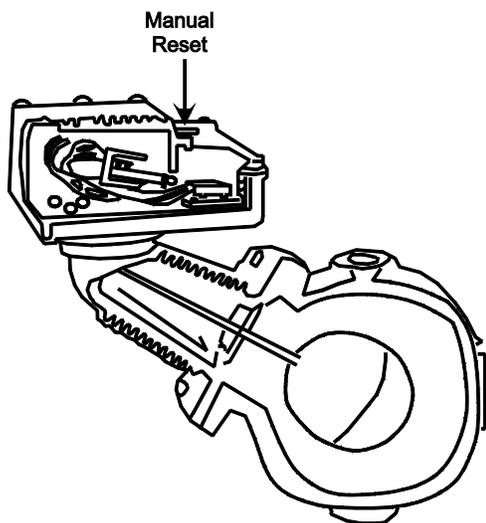
Figure 2. Float Type LWFCO With Manual Reset.
