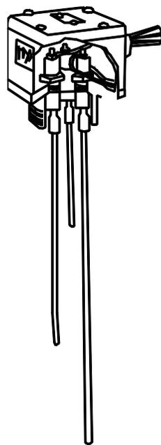
**Figure 4.** Probe-Type LWFCO.
