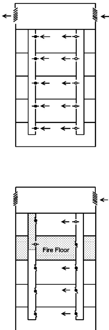
Figure 5. Heat And Smoke Venting Using The HVAC System.
