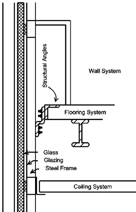
Figure 3. Glass In Metal Frame Curtain Wall.
