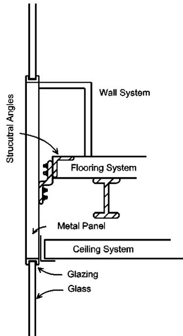
Figure 4. Glass And Metal Panel Curtain Wall.
