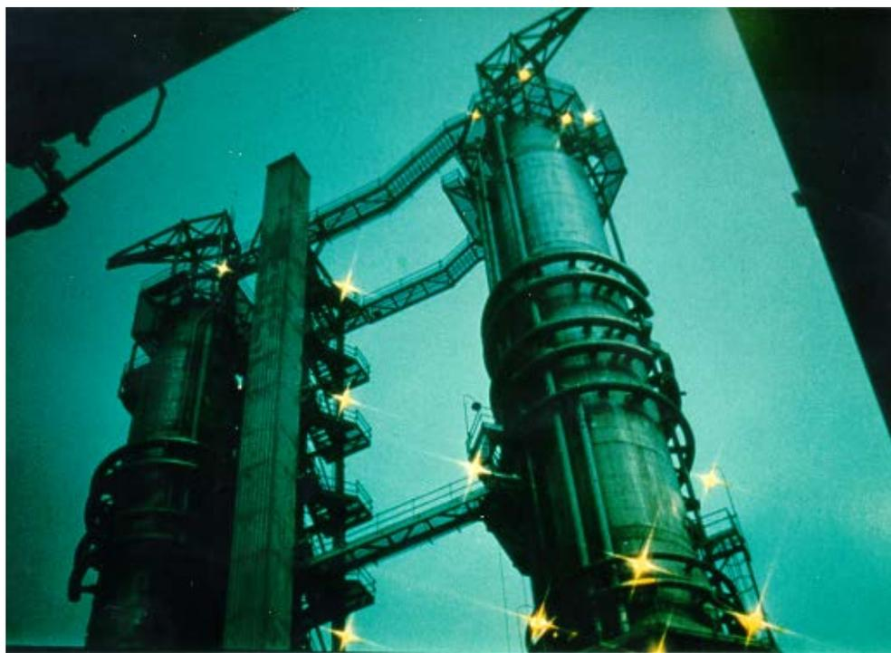
**Figure 6.** Continuous Digesters
