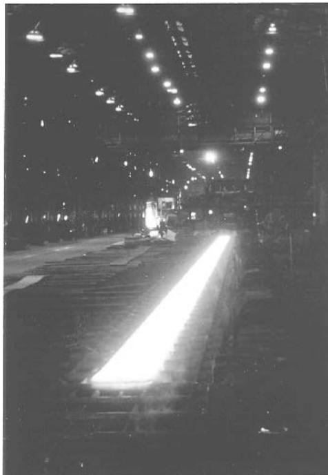
**Figure 9.** Hot Slab On The Run-Out Table From A Single Stand, Reversing Hot Mill (in background).
