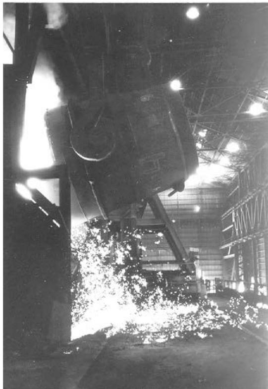
Figure 6. Pouring From A Basic Oxygen Furnace.
