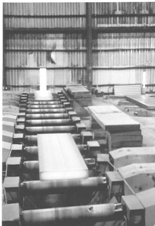
Figure 8. Cut Slab From Continuous Caster.
