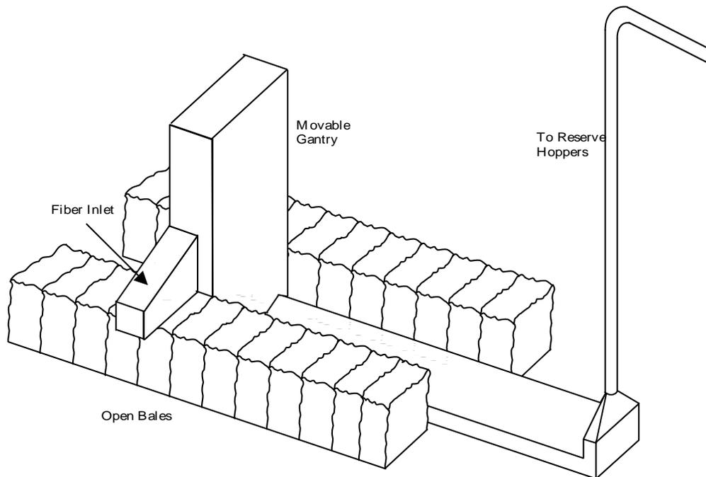
**Figure 2.** Typical Automated Bale Opener.
