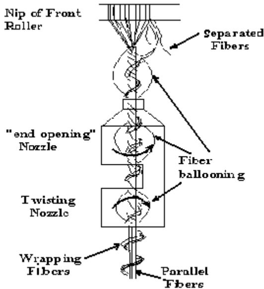
Figure 7. Air-Jet Spinning.
