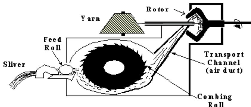
Figure 6. Rotor Spinning.
