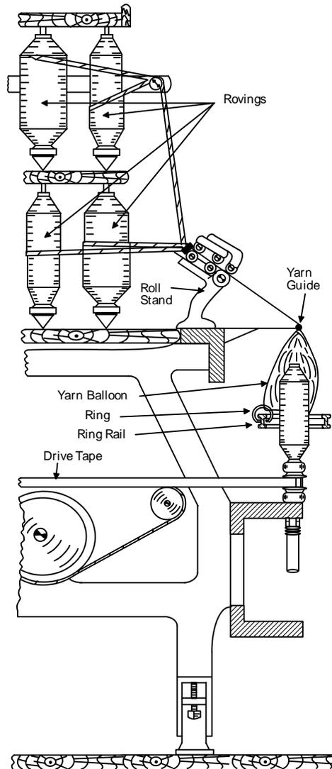
Figure 5. Ring Spinning Frame.
