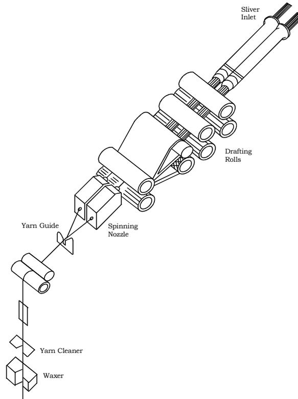
**Figure 8.** Dual Air-Jet Spinning.
