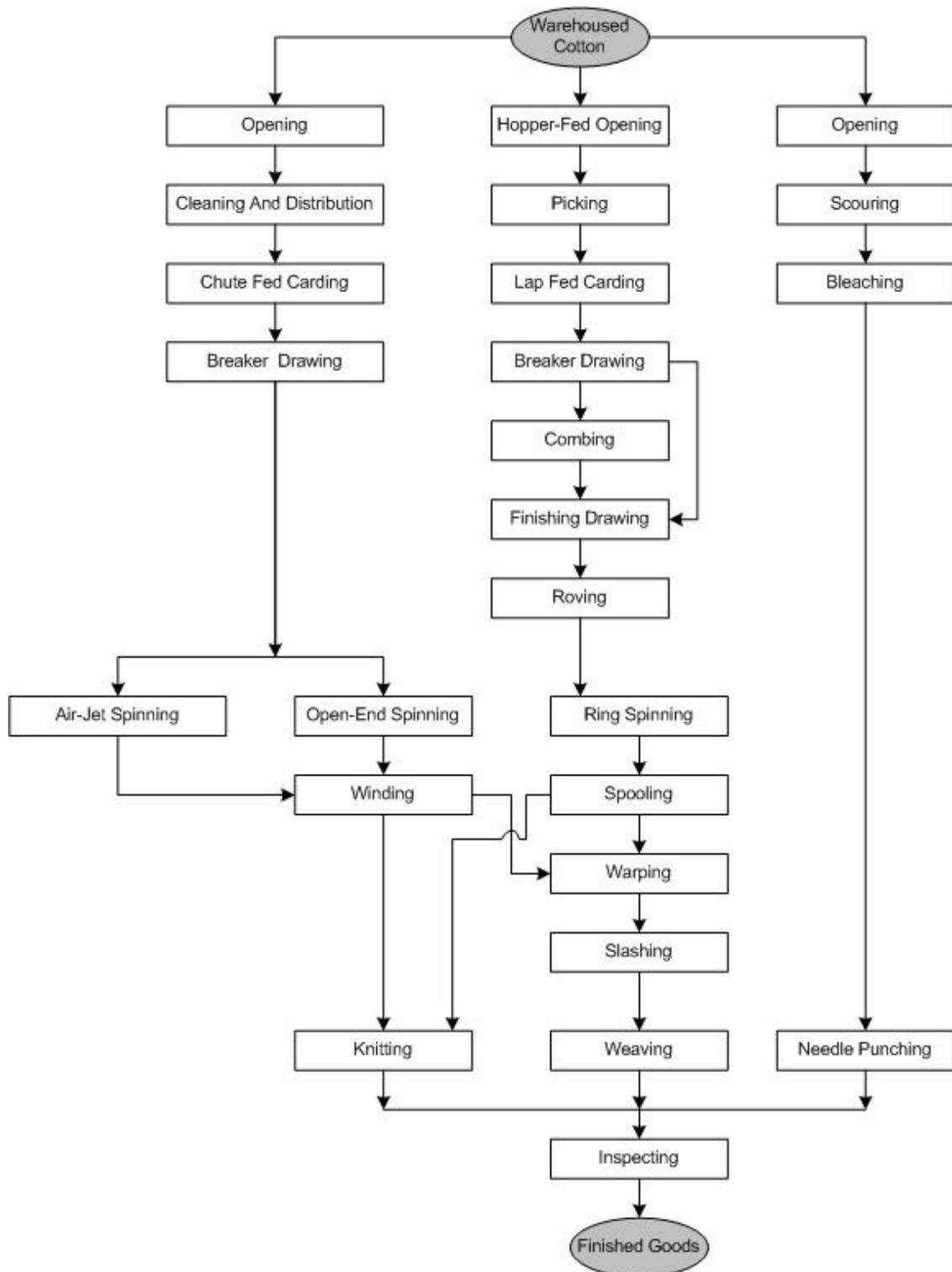
Figure 1. Flow Chart For Manufacturing Cotton Fabric.
