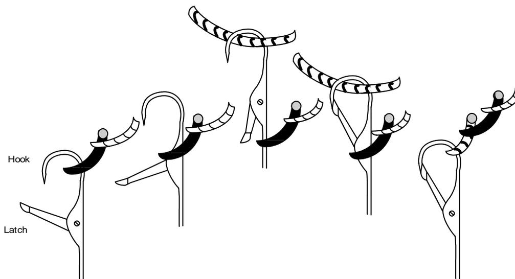
Figure 9. Operation Of An Automatic Knitting Machine.
