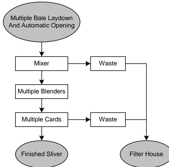
Figure 3. Details Of Modern Opening And Blending Operation.
