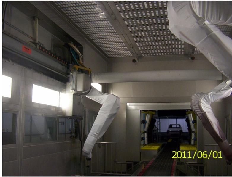
**Figure 4.** Electrostatic Painting Operation.
