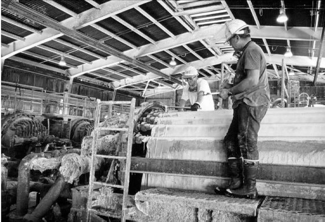
**Figure 2.** Filter Room Showing Two Filters Closed (Left Background) And One Open (Right).
