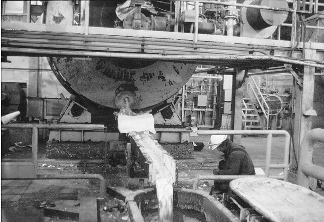
Figure 3. Aluminum Ingot Casting.
