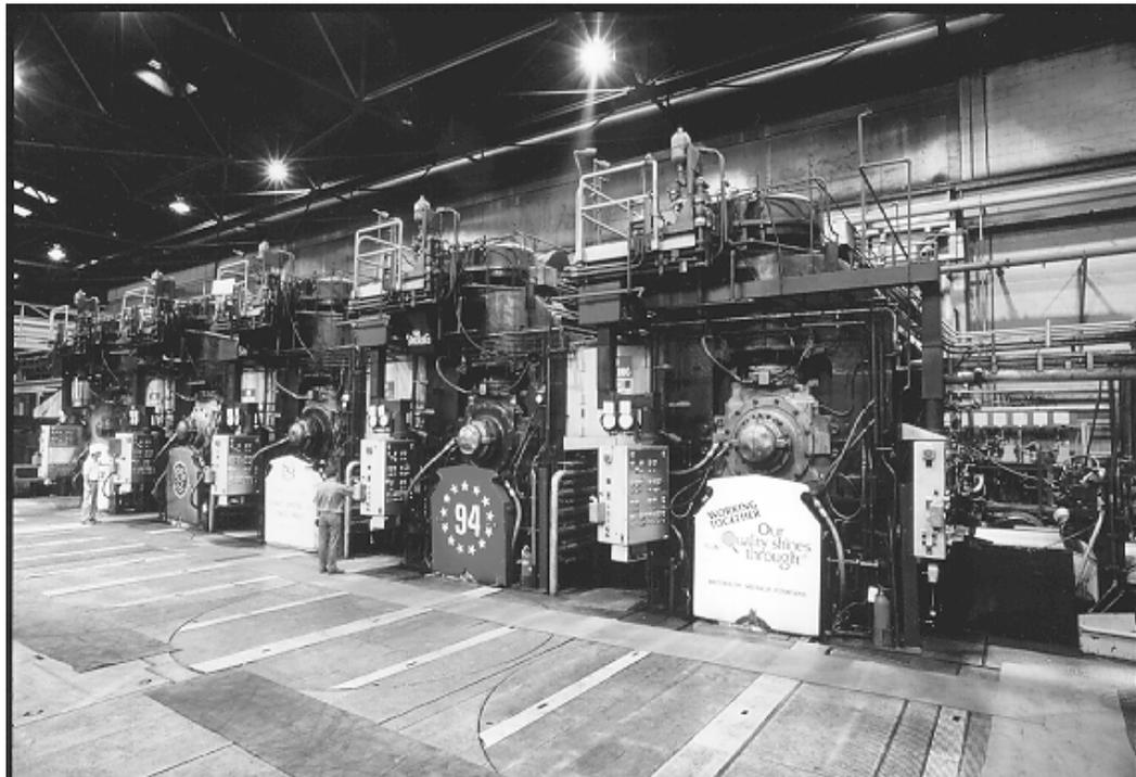
Figure 7. A 5-Stand Aluminum Cold Rolling Mill.
