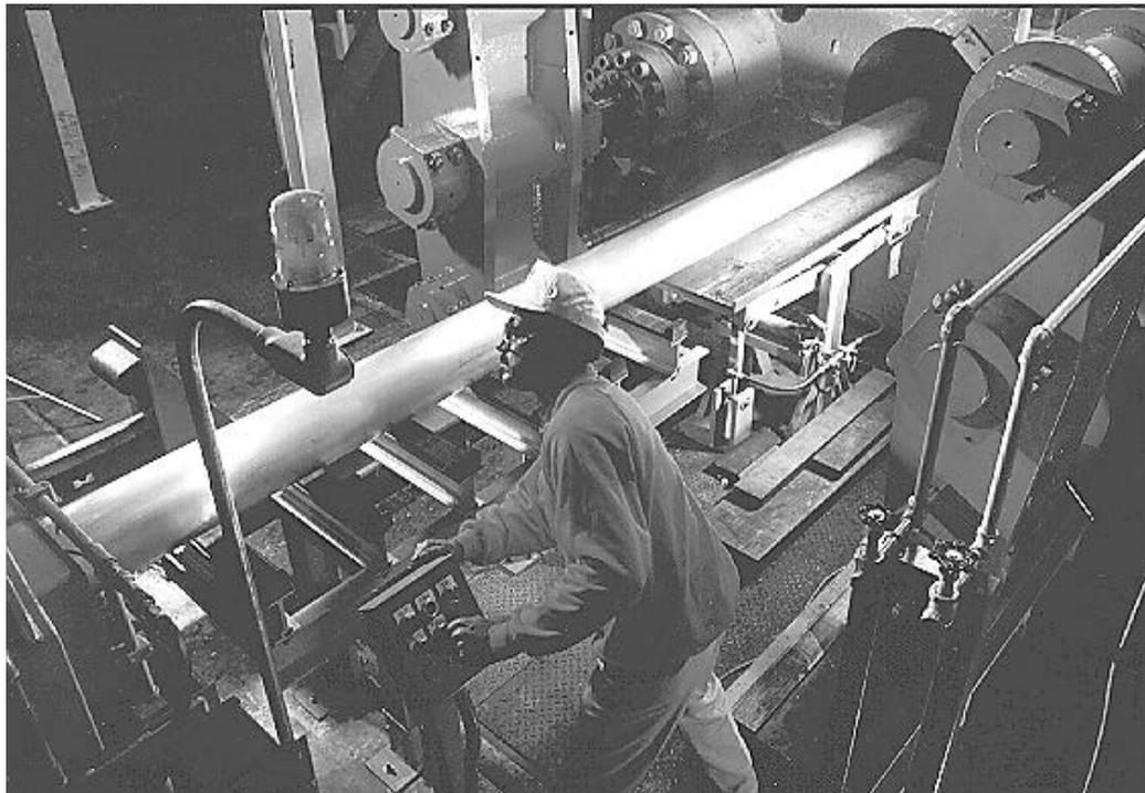
**Figure 6.** An Aluminum Extrusion Press.
