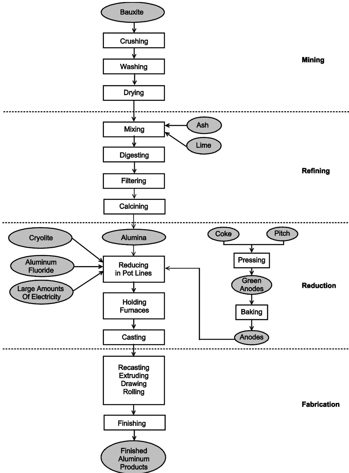
Figure 1. Simplified Process Flow From Aluminum Ore To Finished Aluminum Products.
