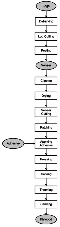
Figure 1. Flow Chart For Plywood Manufacturing.
