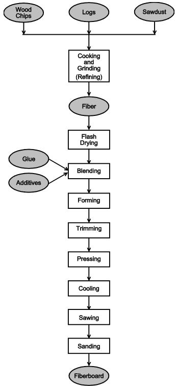
Figure 3. Flow Chart For Manufacturing Fiberboard.
