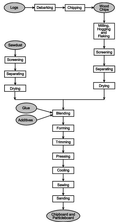
Figure 2. Flow Chart For Manufacturing Chipboard And Particleboard.
