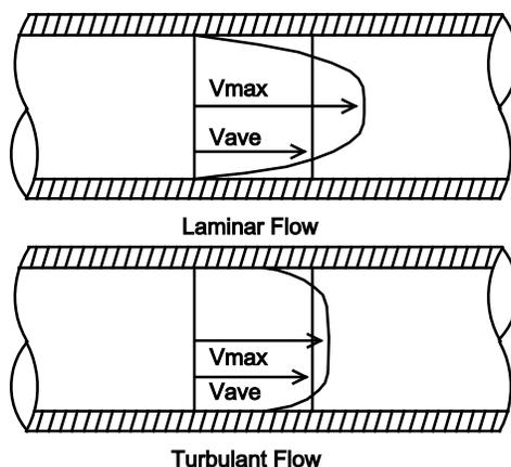
Figure 4. Typical Pipe Velocity Profile.
